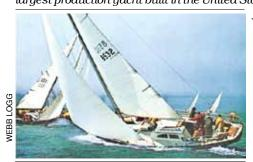
fact that the 50s displaced 32,000 lbs and were built before the oil crisis of 1971, their hulls are nearly an inch thick of solid fiberglass. Sixty-two 50s were built between 1965 and 1972. Perhaps the most famous was Steve and
