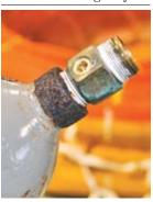
The necks of inflation cylinders can corrode if wet.
