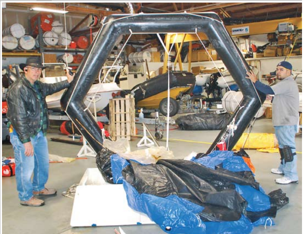
A tale of two liferafts — Clockwise from bottom, it only took Sal (left) and his crew about 10 minutes to turn our raft into a donut; the seams were so bad you could poke a hole in them with your finger; (center) the PVC raft had a number of leaks, as evidenced by the bubbling soapy water; the top tube just pulled right off; the Toyo's zippers were unusable; the Toyo stayed inflated but was still condemned, while the Bombard was just a mess; the burrito; the white PVC case allowed UV to break down the raft hidden inside. Scary!
