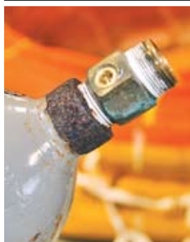
The necks of inflation cylinders can corrode if wet.
