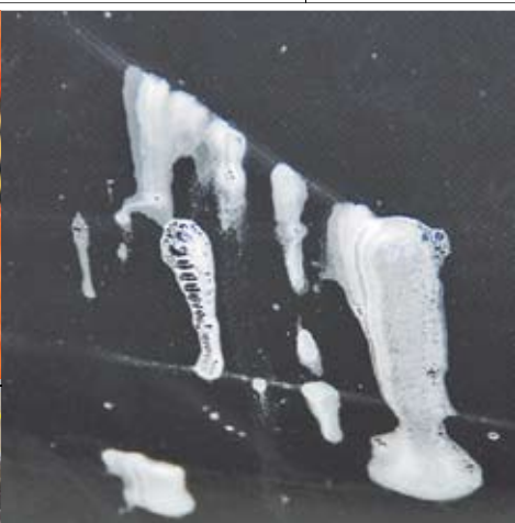
A tale of two liferafts — Clockwise from bottom, it only took Sal (left) and his crew about 10 minutes to turn our raft into a donut; the seams were so bad you could poke a hole in them with your finger; (center) the PVC raft had a number of leaks, as evidenced by the bubbling soapy water; the top tube just pulled right off; the Toyo's zippers were unusable; the Toyo stayed inflated but was still condemned, while the Bombard was just a mess; the burrito; the white PVC case allowed UV to break down the raft hidden inside. Scary!
