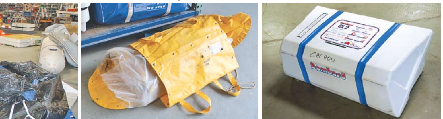
A tale of two liferafts — Clockwise from bottom, it only took Sal (left) and his crew about 10 minutes to turn our raft into a donut; the seams were so bad you could poke a hole in them with your finger; (center) the PVC raft had a number of leaks, as evidenced by the bubbling soapy water; the top tube just pulled right off; the Toyo's zippers were unusable; the Toyo stayed inflated but was still condemned, while the Bombard was just a mess; the burrito; the white PVC case allowed UV to break down the raft hidden inside. Scary!
